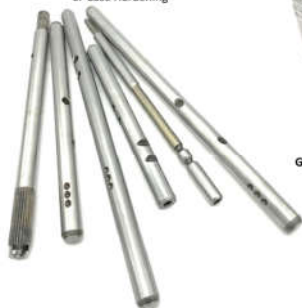
Gear Shift Shaft for Heavy Transmission Material: C45 or 42CrMoS4 Range: Ø16-32mm Extra: Grinding + Polishing + Induction Hardening or Case Hardening
